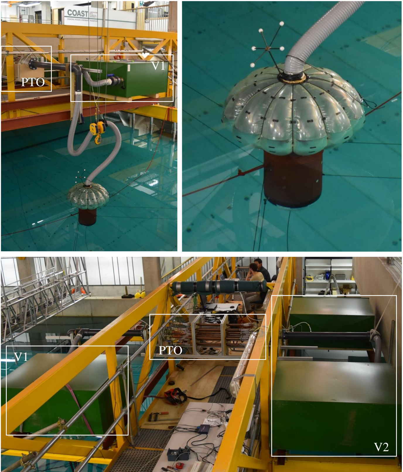
Fig. 3 Photographs of the test setup and model of device A in the wave basin
