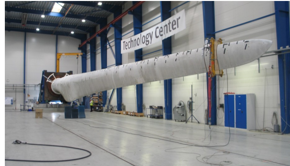
Figure 2: The 37.3m wind turbine blade in the experimental setup; the pulling clamp is mounted near the tip; the RF absorbers are visible at mid-way to the root.
