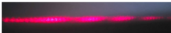
(a) Image of a fringe pattern projected onto a piece of black cardboard. The fringes are seen as periodic small bright spots occurring on a background of larger intensity variations.
