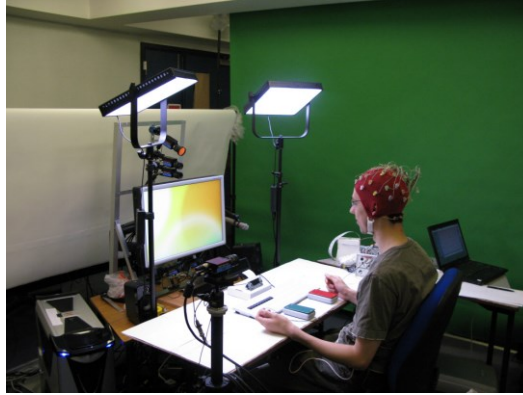
Figure 1-1 A scenario in laboratory environment for physiological signal acquisition aimed at automatic health monitoring (obtained from [20]).
