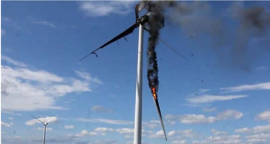
Fig. 1.4. A falling blade with fire in US, 23 July 2015 [Reproduced with permission from Kimberly Watley, Copyright 2016, Kimberly Watley], [7].
