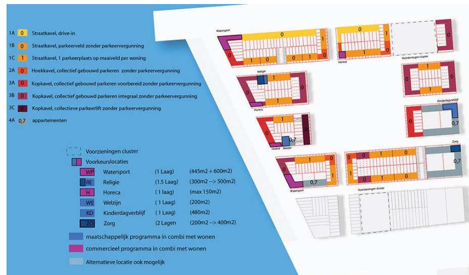
Figure 8. The image shows the preliminary concept plan for the Western part of centrum eiland, the organization of the self-built plots, the expected planning of services within the grid and the different typologies of houses in relation with parking
