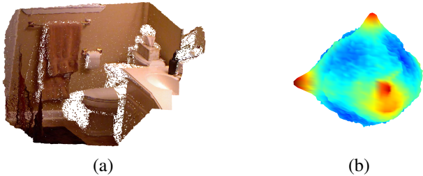
Fig. 4. (a) Shows a scene plotted in 3D Cartesian coordinates, besides it, in (b) a plot of the concentration of normals is shown, it is created using a histogram of the normals, where the concentrations are plotted as elevations on a sphere, corresponding to the direction of the normals. Notice the three main bulges (red color), they correspond to the three dominant normal directions in the image.
