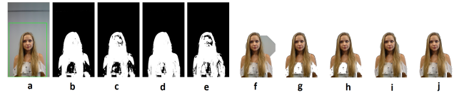
Fig. 5. (a) Original image with a ROI and (b)-(e) obtained masks from image pairs. Then, obtained results with Grabcut: (f) Region of Interest, (g) Parallel Fusion, (h) Parallel Fusion with Weights, (i) Parallel Votes, (j) Parallel Votes with Weights.
