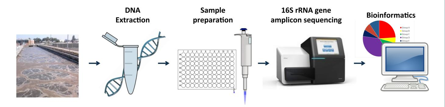
MiDAS<sup>1</sup> provides protocols for DNA extraction, 16S rRNA gene amplicon library preparation<sup>2</sup> and bioinformatic analysis – all optimised for application to wastewater treatment system samples.
