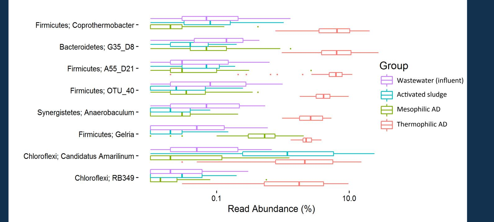
**MiDAS** includes abundance values for influent wastewater, activated sludge and anaerobic digester (AD) – identifying abundant phylotypes and giving an insight into migration. An important example being the link between foaming episodes in anaerobic digesters and migration of "Ca. Microthrix spp." from activated sludge.
