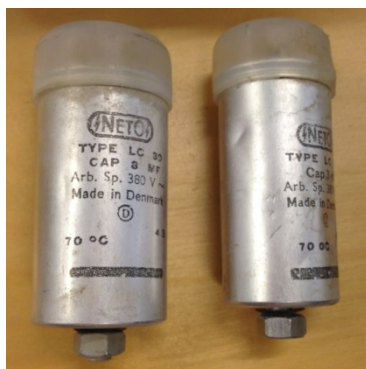
Figure 2.3 Danish fluorescent light ballasts with a PCB congener composition similar to Aroclor 1248.
