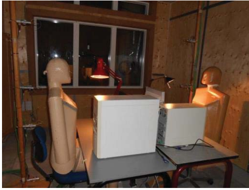
Fig.3. The test chamber with an office layout
