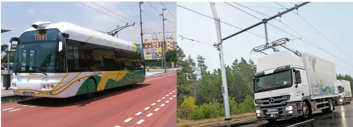
Figure 6: Siemens trolley bus [32] and eHighway hybrid truck which can both be powered by electricity delivered via overhead lines [33]: © Siemens press picture (reused with permission).
