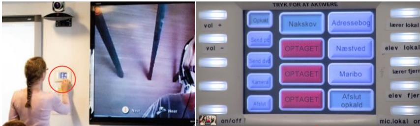
Figure 13: The control panel for the videoconference.
