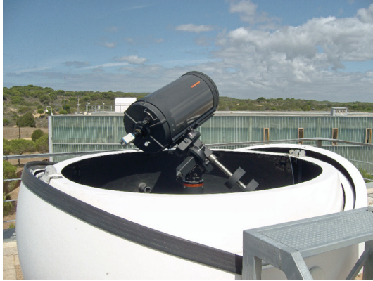
FIGURE 3: Image of one of the two 14-inch SC telescopes integrating the impact flashes detection system.
