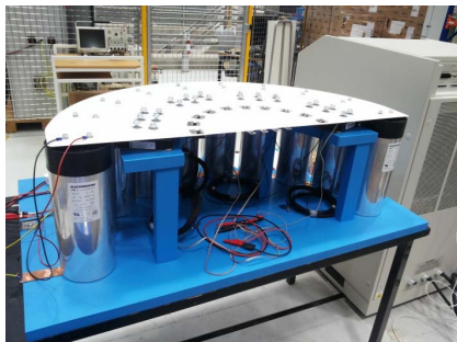
Fig. 6. Non-destructive test short-circuit setup for power modules [24].
