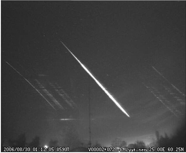
Figure 4. Fireball spectrum of the 2006 August 30 bolide. A diffraction grating of 1000 grooves \text{mm}^{-1} was used.
