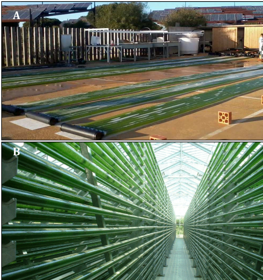
Figure I.10. Tubular photobioreactor systems. (A) Horizontal tubular photobioreactor, CIECEM, Huelva (Spain). (B) Vertical tubular photobioreactor, California Polytechnic State University, California (USA). http://brae.calpoly.edu/CEAE/images/biofuels3.gif
