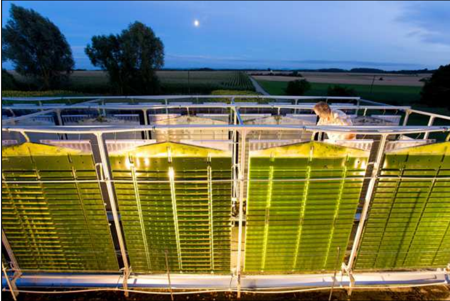
Figure I.11. Flat panel bioreactor. Source: http://www.esru.strath.ac.uk/EandE/Web_sites/09-10/ZeroCarbonCommunities/Algaehome.html
