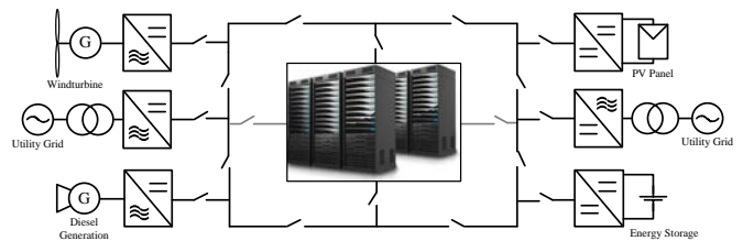
Fig. 2. Ring-bus based DC microgrid feeding critical load.
