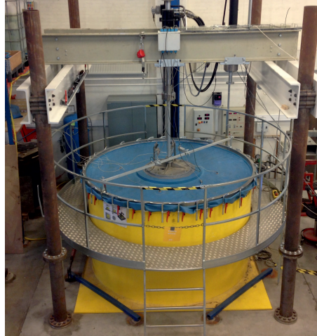
Figure 2.1 A test set-up for the axial bucket foundation testing with an applied overburden pressure.
