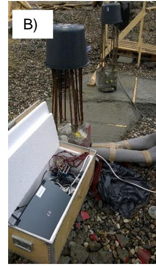
Figure 20: A) Ongoing TRT of the 16 m long EP at Rosborg North. Inlet- and outlet pipes are insulated to prevent disturbances from ambient conditions. B) The adjacent box, covered by black plastic bags contains the computer and the modules to log the temperature data from the Pt100 temperature sensors casted into the pile (see Figure 10).
