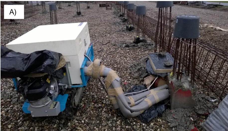
Figure 20: A) Ongoing TRT of the 16 m long EP at Rosborg North. Inlet- and outlet pipes are insulated to prevent disturbances from ambient conditions. B) The adjacent box, covered by black plastic bags contains the computer and the modules to log the temperature data from the Pt100 temperature sensors casted into the pile (see Figure 10).
