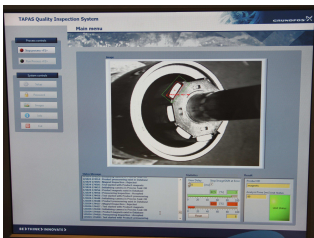
Fig. 1. Vision detection system in execution mode.
