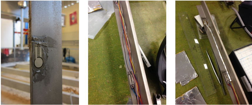
Figure E.2: FlexiForce sensor mounted on the steel bar with the wiring led to the backside of the bar.
