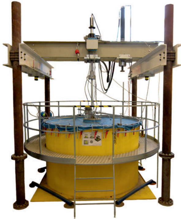
Figure C.2: Setup for a test with applied suction.
