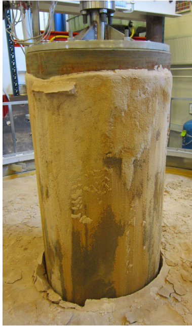
Figure C.5: Uninstallation of the pile after a test with applied suction. Sand is not resaturated before uninstallation, and some sand is stuck to the upper one third of the pile.
