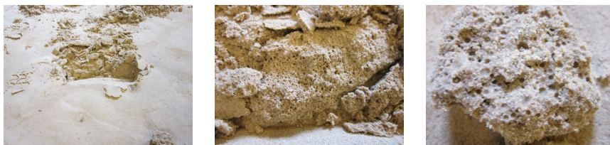
Figure 4.5: Sand structure after tests with applied suction.
