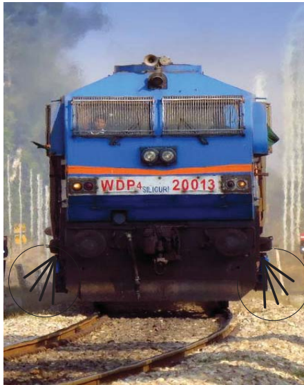
Figure 6.2: Rail engine - deployment agent Spraying tubes (encircled)[15]
