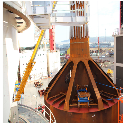
Figure 1.10: Monopod bucket used as foundation for the Mobile Met Mast at Horns Reef II offshore wind farm. (Universal-Foundation 2015)
