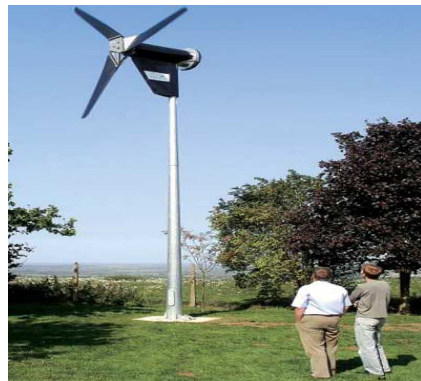
Figure 1.4: Proven 6Kw wind turbine at Brill school. (RET 2015)
