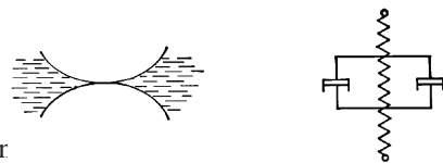
Figure 2.13: Schematic representation of the region of contact between grains with viscous fluid and the corresponding spring-dashpot model (Biot 1962b).
