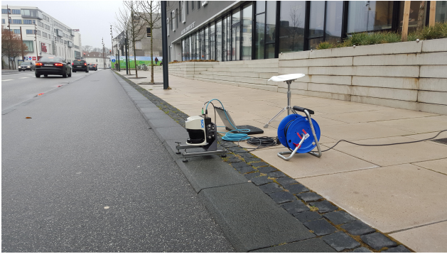
Figure 3: A view of the temporary sensor setup at the roadside. On this picture, only the horizontal scanner is mounted. A bike path runs between the sensor and the road.
