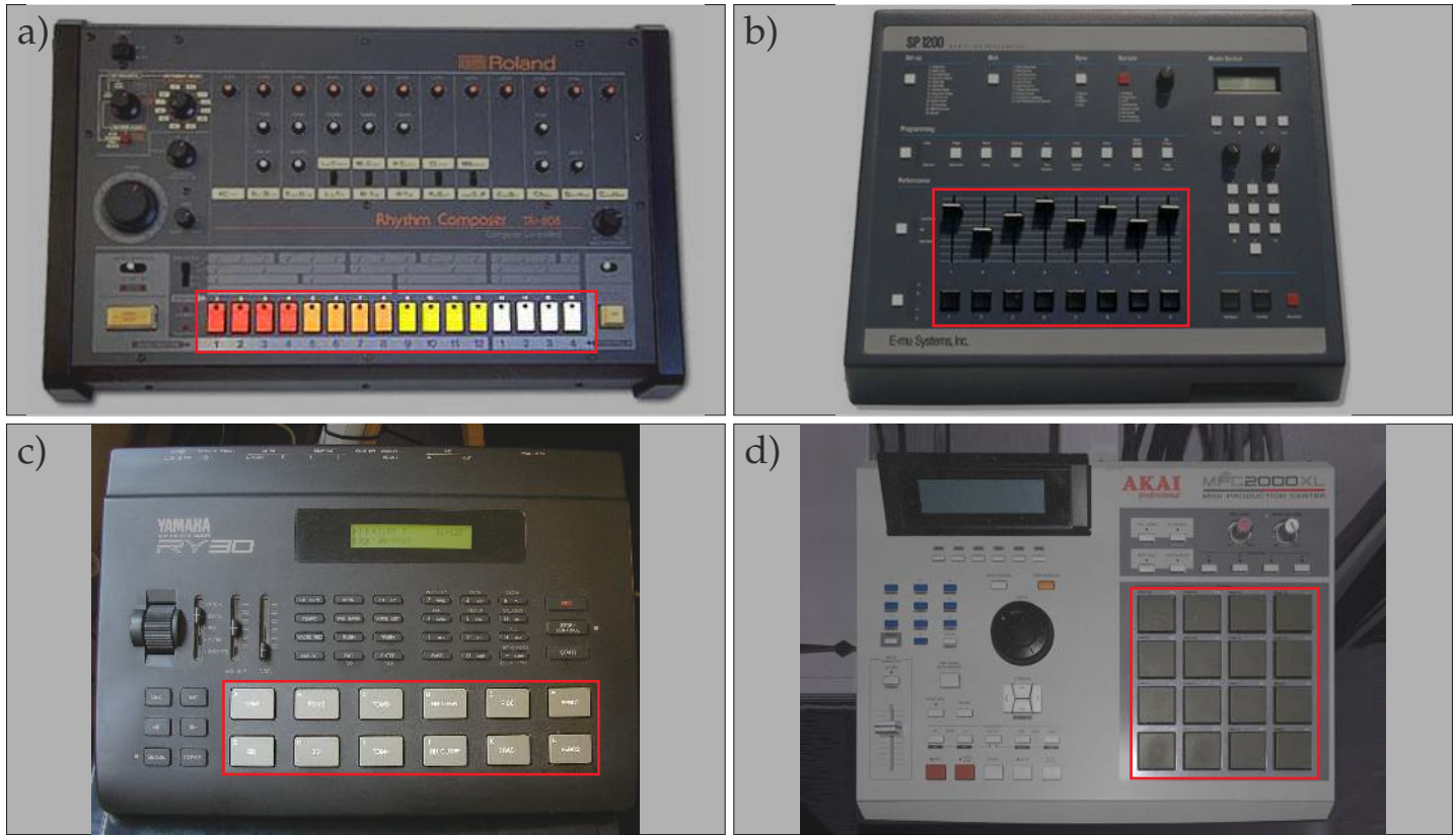
Fig. 3.1: Some classic rhythm/drum machines, with key user interface components: a) Roland TR-808, with step sequencer indicated; b) E-mu SP 1200, ibid. ; c) Yamaha RY30, with "pad bank" indicated; d) Akai MPC2000, ibid. (from ref. [53])
