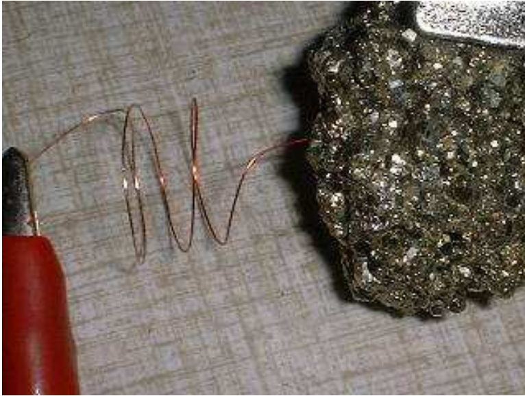
Fig. 4.2: Harkening back to simpler times, when bare rock and metal were enough to form a relevant electronic device (here a negative resistance tunnel diode; ref. [144]).
