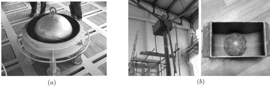
Figure 3.2 Previous investigations of the roller damper. (a) The ball vibration absorber used on two TV towers (Pirner 1994). (b) Shaking table tests on the performance of roller dampers for controlling wind turbine tower vibrations (Zhang et al. 2014).
