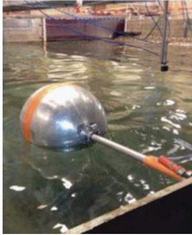
Fig. 6. Scaled model of the GyroPTO point absorber being tested in a wave tank.
