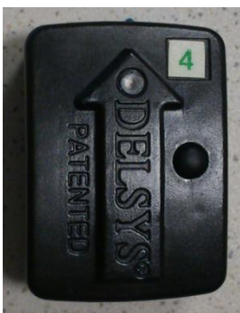
Figure 32: EMG wireless sensors
