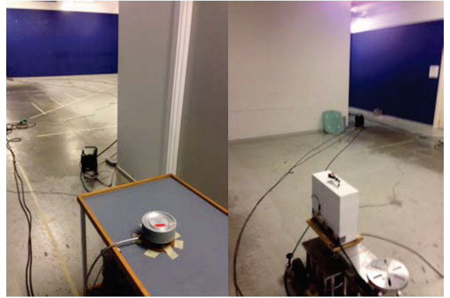
Fig. 2. Large empty room, NLOS measurement a) Tx viewpoint towards Rx b) Rx viewpoint towards Tx
