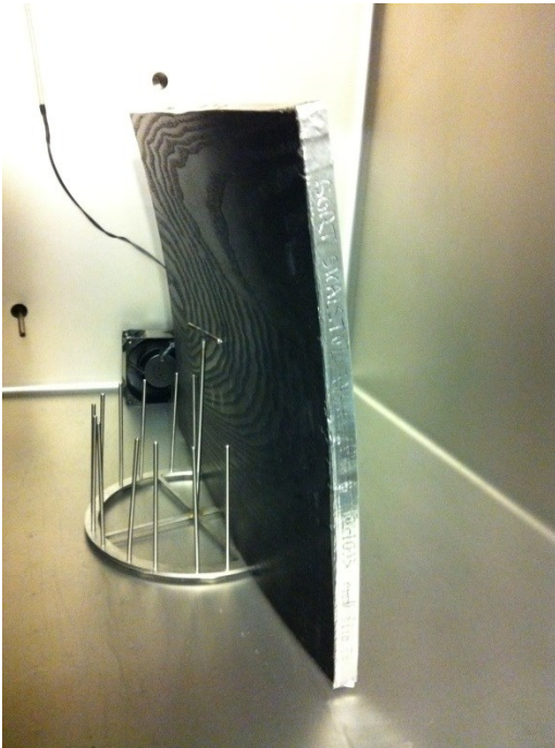
FIGURE 1. KITCHEN FRONT DOOR, CUT TO SIZE AND WITH SEALED EDGES, IN A 0.225 M 3 CHAMBER.
