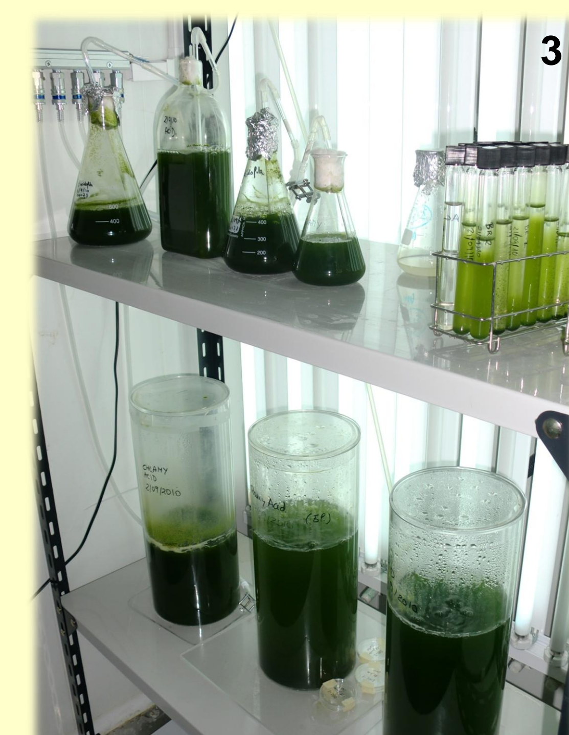
Figures 2 and 3. Tubular bioreactor, air fluidized-bed bioreactors and conical flasks erlenmeyers used in the experiments.
