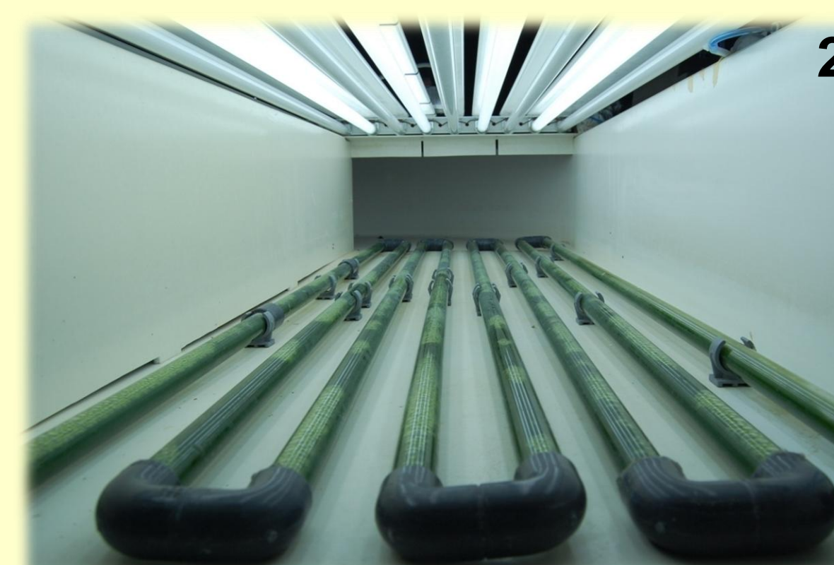
Figures 2 and 3. Tubular bioreactor, air fluidized-bed bioreactors and conical flasks erlenmeyers used in the experiments.
