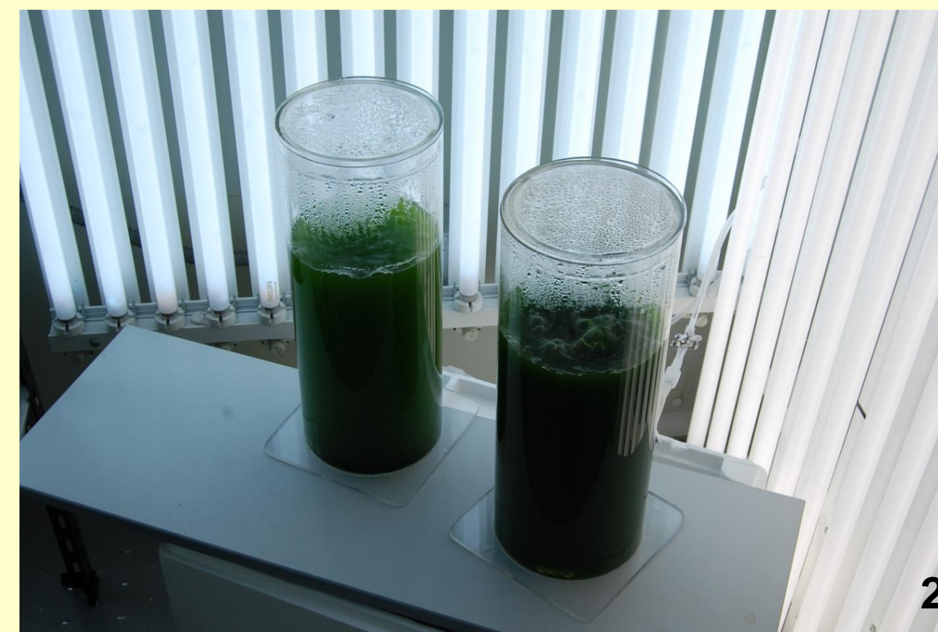
Figure 2. Air fluidized-bed bioreactors used in the biomass productivity experiments.
