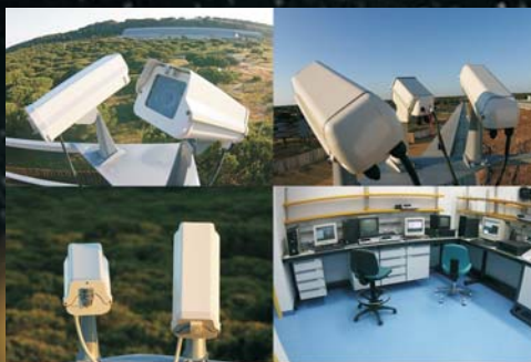
Figure 2. Images of the control room and some of the high sensitivity CCD video cameras of the CIECEM meteor observing station.
