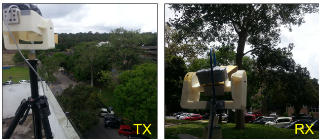
Fig. 1. Directional measurement setup with TX antenna deployed above rooftop illuminating the densely-vegetated area of interest, and RX antenna mounted on a rotating pedestal close to street level.
