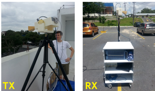
Fig. 1. Directional measurement setup with TX antenna on a tripod with fixed orientation, and RX antenna mounted on a semi-automated rotating pedestal.
