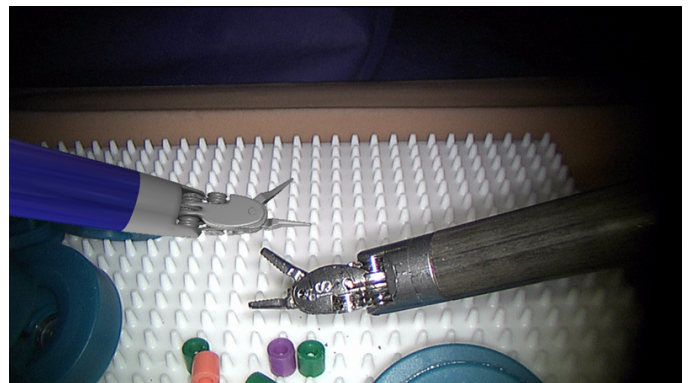
Fig. 6. Endoscopic video signal overlaid with a virtual instrument (blue) in real-time. This composition is shown to the left eye. A similar image is shown to the right eye, but with the real and virtual camera offset to the right.
