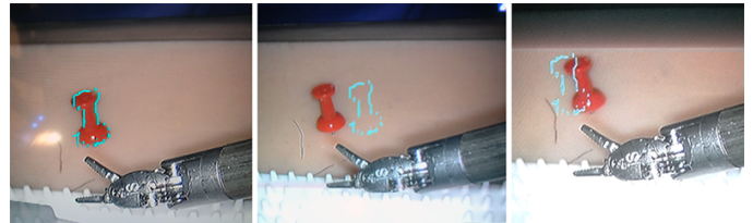
Fig. 2. Telestration. Left: drawing around a pen on the touch screen. Center: the drawing as displayed in the surgeon console’s left display. Right: the drawing in the right display. The drawing gets offset for both eyes, making it appear at a different depth than the background. For some users this creates double vision and thus makes precise pointing impossible.
