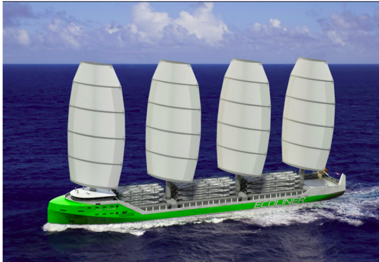
Figure 2 A sketch of a sailing Ecoliner vessel. Source: Dykstra Naval Architects (2013)
