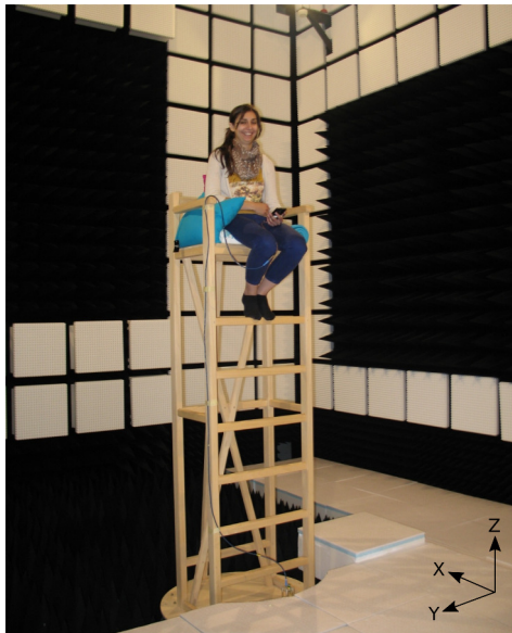
Fig. 1: User in the measurement chair inside the anechoic room. The reference coordinate systems is also shown.
