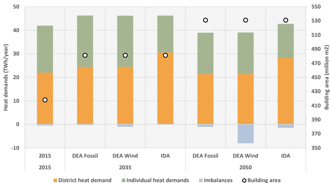
Figure 43: Heat demands and heating imbalances along with the building area in the 2015, 2035 and 2050 scenarios
