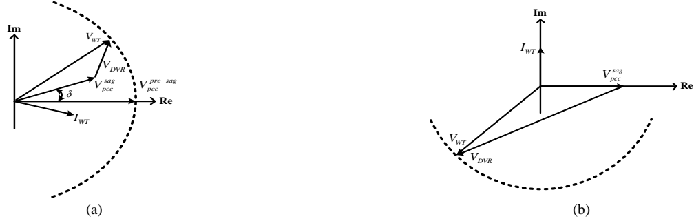
Fig. 9. Single-phase vector diagram. (a) Voltage dip compensation with DVR. (b) Voltage dip compensation once the phasor has been rotated.
