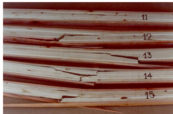
Figure 5. Series of mixed poplar-eucalyptus beams after the bending test (photo by G. Castro).
