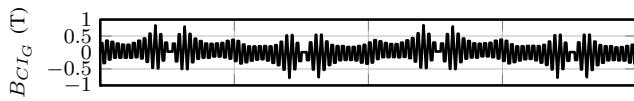
Fig. 12. Simulation results. (a) Flux density waveform in the coupled inductor that is used to suppress the circulating current between the high side and the low side converter group.
