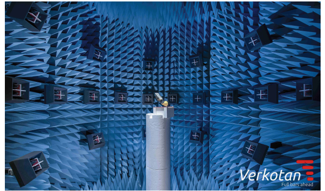
Figure 13. A photo of the practical 3D MPAC setup in the measurement. The chamber size is 6.0 m x 6.0 m x 5.8 m and the distance from the probes to the center is 2.2 m. There are 16 probes in elevation 0^\circ with 22.5^\circ azimuth spacing, 8 probes in elevation +30^\circ with 45^\circ azimuth spacing and 8 probes in elevation -30^\circ with 45^\circ azimuth spacing. There was no azimuth angle offset between the three rings. Note that a Satimo sleeve dipole was used to scan the field in the measurements.
