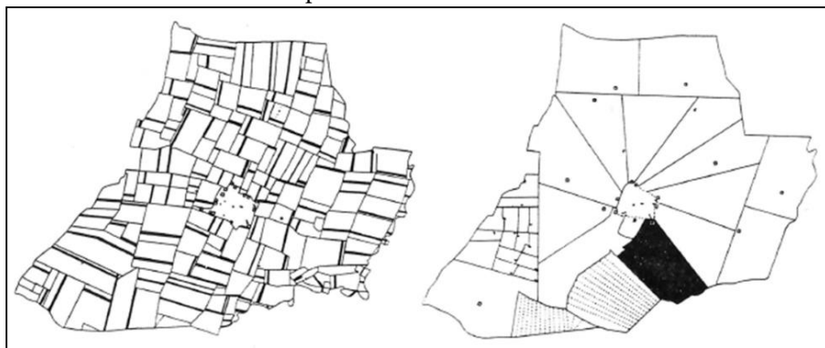
Figure 3.1: Oster Stillinge village near Slagelse before (left) and after land reform (right). Agricultural land belonging in ownership to one agricultural holding enhanced. More than 40 parcels consolidated into one parcel. Source: Østergaard 1967. 25
