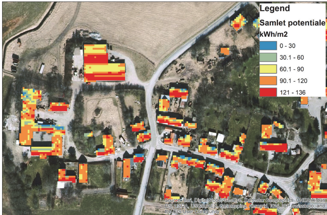
Figure 19: Example of the solar atlas where all roof tops are included
