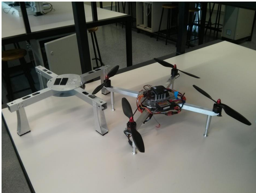
Figure 3. Robot air rescue AirDroneUvic (year 2013-2014)
