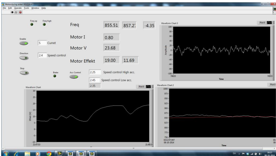
Figure 18. Screenshot from Labview measuring the device performance.
