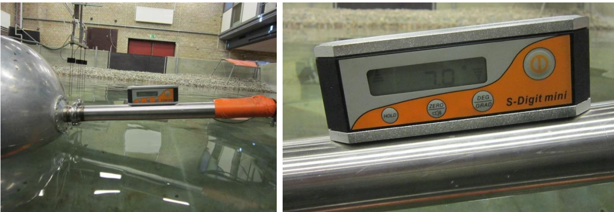
Figure 6: Measured inclination of the device at rest in calm water.
