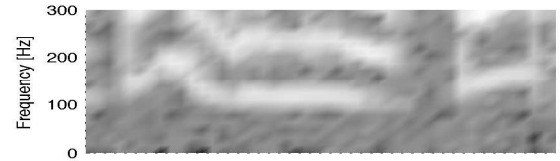
(c) Spectrogram of a speech segment. Note that y-axis is limited to the frequency range containing pitch.
