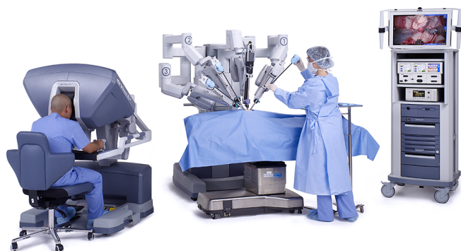
Fig. 1. da Vinci surgery system. Left: surgeon operating the surgeon console. Center: assisting nurse operating the patient cart. Right: vision cart. Copyright 2015 Intuitive Surgical, Inc. [2]
