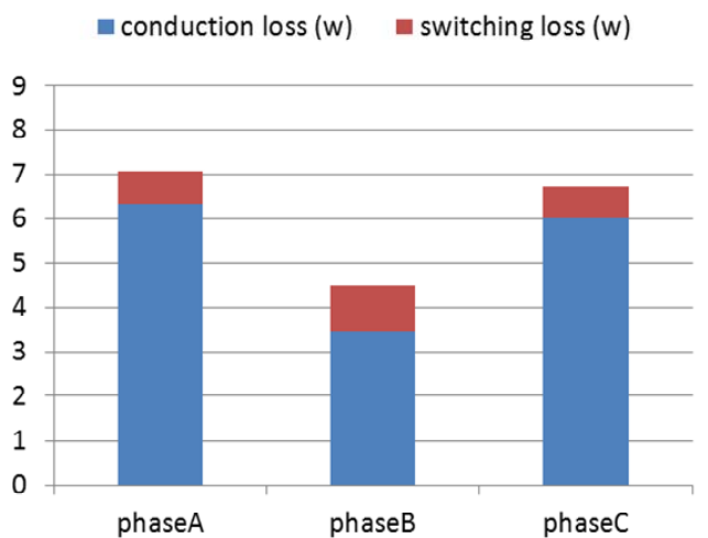
Fig. 13. Experimental per-switch loss distribution of B6 converter when modulated by the discontinuous scheme from (11).
