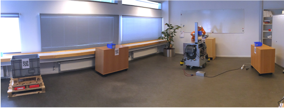
Fig. 9.2.: Environment used for planning experiments, with the feeder on the left, the robot in front of the workstation, the two shelves and four boxes.
